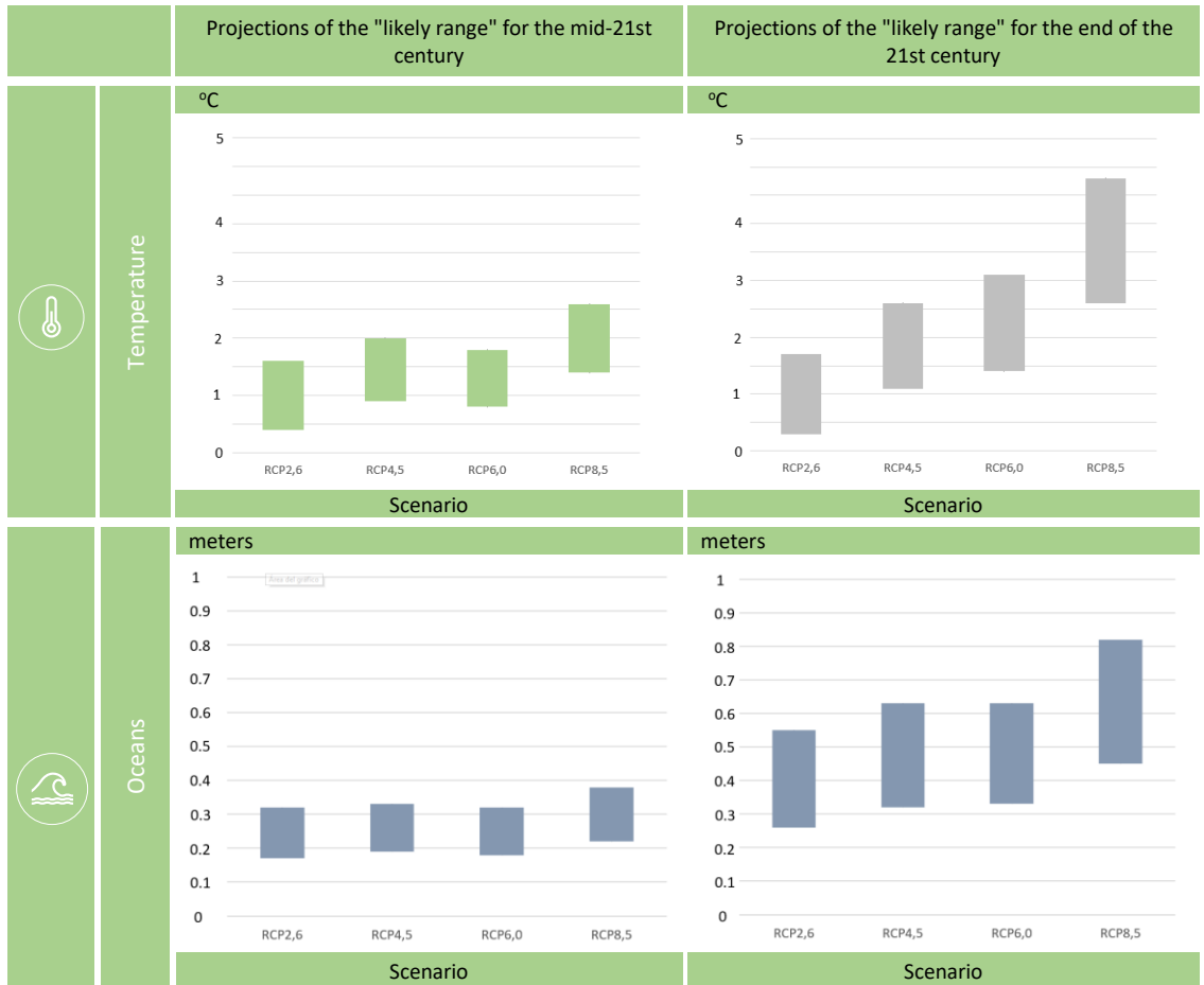
Figure 4-4: "Likely range" projections of global mean surface air temperature and global mean sea level rise for the mid (2046-2065) and late (2081-2100) 21st century, relative to the 1986-2005 reference period. Graph prepared by the author, based on data from the IPCC 2013 report (Stocker, et al., 2013).
